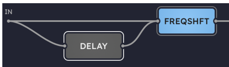
Figure 7: If Thru is on, FREQSHFT will receive two copies of the input signal: one from the IN node, and another passed through the DELAY effect
